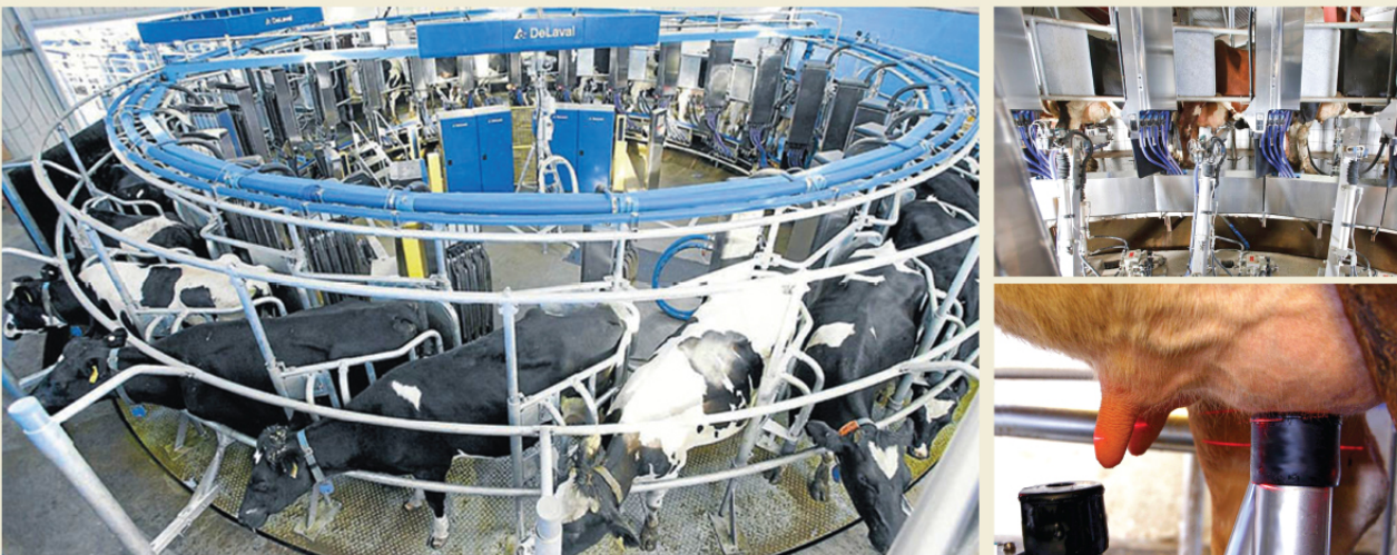
A robotic dairy. The image at top right show three robotic arms that place the cups on the teats. The image at bottom right shows the robotic arm in action as its sensors find the teats before putting the cups on.
